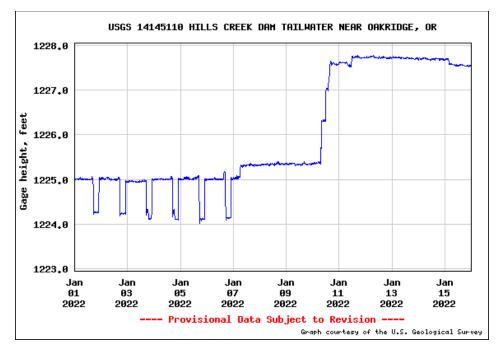
Figure 7. Gage Height (feet); below Hills Creek Dam, Middle Fork Willamette River
